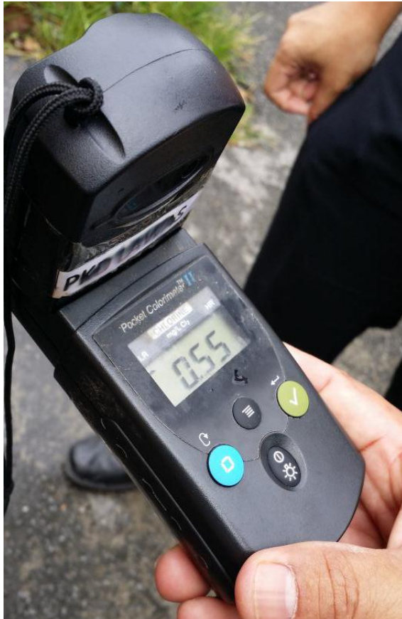
Free chlorine at terminal water 30km away from WTP: 0.55ppm
